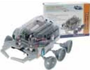
**Scarab** is a robot that uses 2 touch sensors to detect obstacles. When its antennas (touch sensor) detect an obstacle, Scarab will first step back and then automatically execute a two-step manoeuvre to avoid the obstacle.
