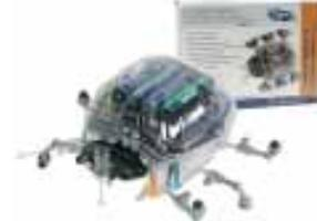
**The Ladybug Robot** walks on 6 legs and uses infrared emitting diodes for "eyes" in order to avoid obstacles. Ladybug walks straight ahead but automatically makes a left turn the moment an obstacle is detected. The Kit comes complete with 2 sets of differently designed legs, which move in their own distinct way. Let the fun begin! Specifications dimensions: 120 x 150 x 85mm (length feelers : 40mm)
